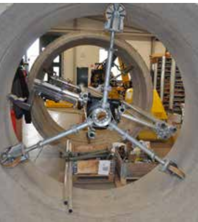
Above, the smallest hydrodemolition system on the market, Jetframe 101 Nalta, launched about three years ago.
